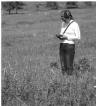
**Figure 9.** Using a hand held Leica SR-20 GPS on site allows precise location of archaeological structures, up to 10 or 20 cm.
