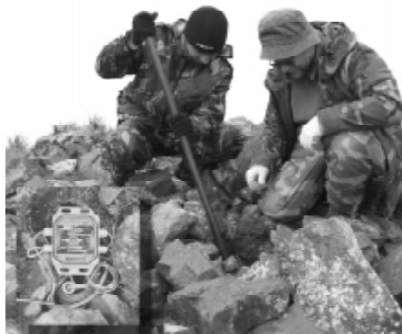
**Figure 29.** Sergei Marchenko at work, implanting data loggers (see detail) at several depths in the surroundings of Scythian burial mounds to monitor the temperature during a full year
