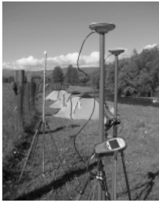
**Figure 6.** The installation of two SR-20 GPS receivers as reference stations in the camp
