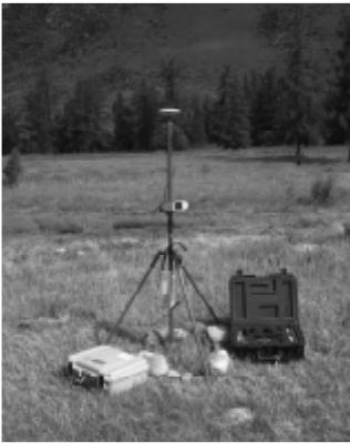
**Figure 7.** When necessary, due to longer distances, the installation of a supplementary C-Nav station in the field is required
