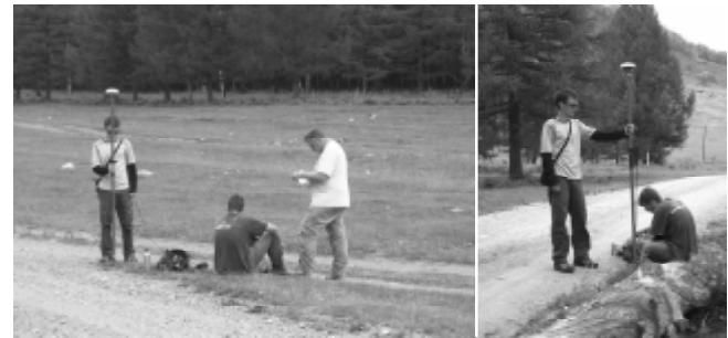
**Figure 3 and 4.** Measuring GCP's with the C&C Technologies C-NAV differential GPS receiver
